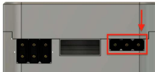
**For Spektrum** radios use the Spektrum port to connect the telemetry output of the receiver to the TTU+.
