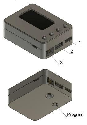
The device has a OLED 128x64 screen and 4 buttons on the front.
