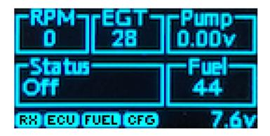
RX icon Is the status of the radio signal, when on, it means that TTU+
