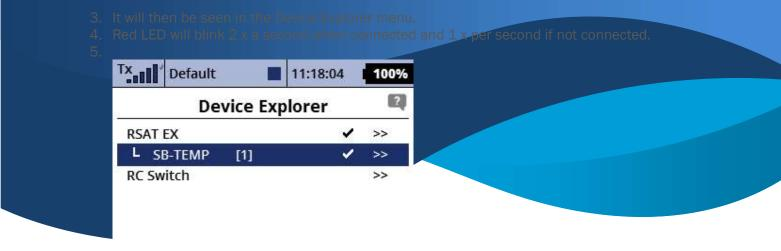
7. Connect the K type sensors tot he corensponding ports en enable them, if you have a port that has NO sensor connected please disable it otherwise you can get false readings!
