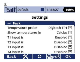
9. Selecting Temp probe , make sure SB-temp Temp probe is set to TP1 its the only one enabled at the moment , more will be supported in the future.
