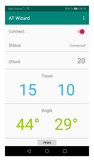
The AT Wizard will switch off after disconnect (connect slider) or closing the app and disable the bluetooth connection. This will take 30 seconds..
