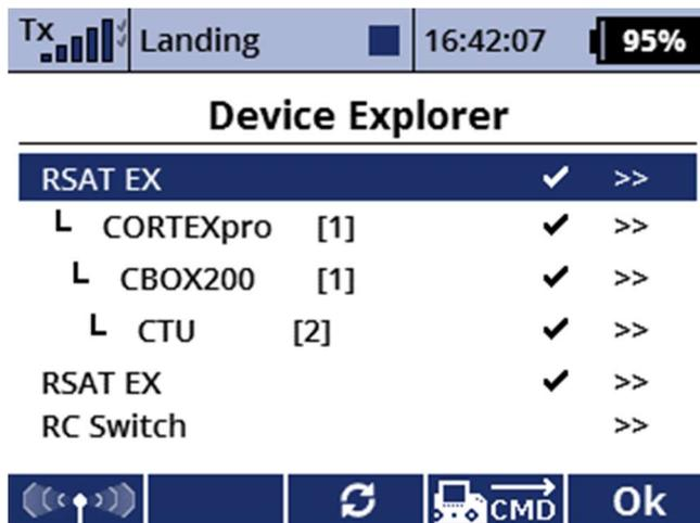
**Make sure the CTU is connected to a EX input on the Jeti receiver and that the port is configured for EX.**
