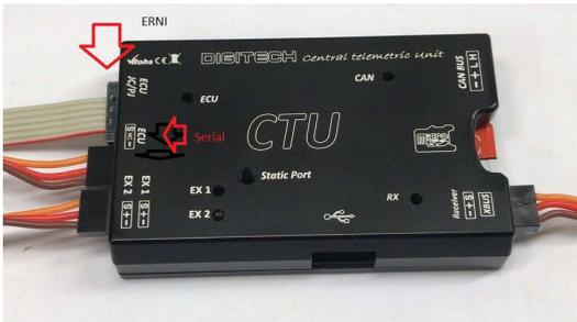
**Erni / JP/JC** This connector goes either to the Jetcat ECU direct or thru the DSP-CTU1/2 Adaptor. (Fadec or Jetcat V6 ECU or Projet)
